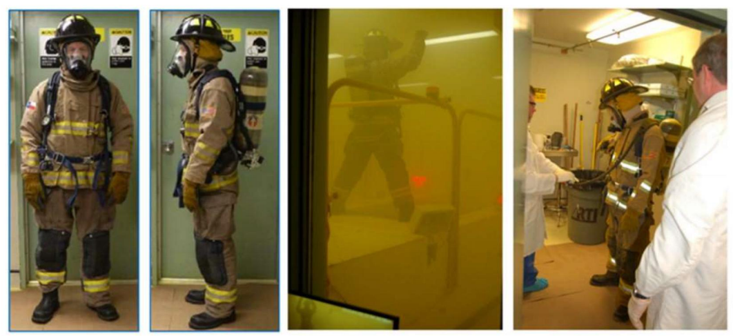
Photo: Testing process for florescent aerosol screening
